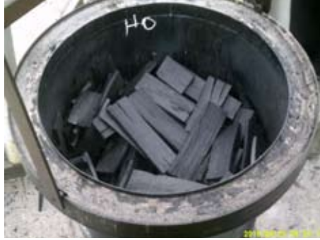
Houtafval in de potten vóór en na carbonisatie. (foto's: Environmental Services & Support NV)
